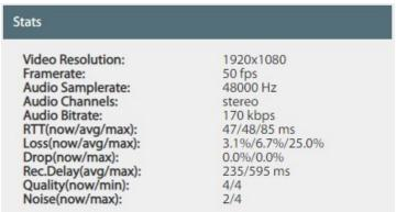
The statistical values of the SRT connection are created every second, and we explain them below: *RTT*: it is the ping in the current second, the average ping in the last hour and the maximum ping in the last hour.
