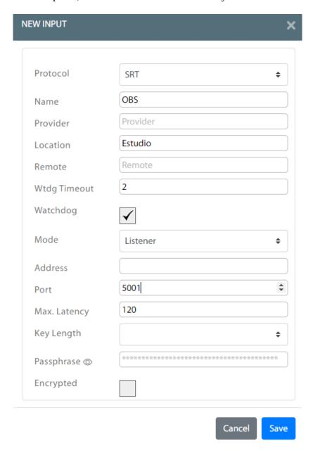
In Name we set OBS to identify the origin of the video for this INPUT, though we could have set any other descriptive name that helps us identify it easily in the panel.
