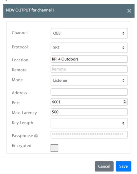
We will only comment on the Port value, which to simplify we used 600x for the OUTPUT numbered incrementally as we create them (though this is not mandatory). If by chance we use a port that is already being used in another Listener connection in the server, the system will warn us to change it to another one, so there is nothing to worry about. Click on Save, and we will have to click on the black triangle icon of the INPUT to see the new created OUTPUT.
